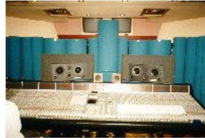
The Dierks Studio in Cologne, was very similar except that there was space on either side of the SSL to place Studio Traps and complete the ATTACK Wall. Swedien has one of the best mic techniques in the industry and as an engineer, Swedien does not just record a signal - he works with spaces, resulting in a more emotional recording. With the ATTACK Wall he was able to hear and see the spaces. His masterful work was an eye opener for all the participants.
